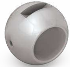
3 mm relief hole face the upstream
